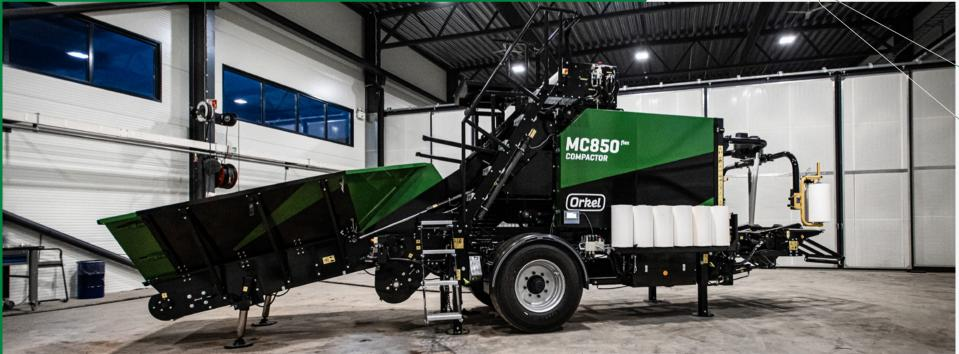
The weight of a flex bale starts at approximately 100 kg, and may range up to 450 kg, according to customer preference. Compared to the initial MC850 model, the MC850 flex model is equipped with a kit and specialized bale settings, limiting the bale diameter to 50 cm. Furthermore, the compactor's wrapper unit is re-sized to fit a 200 - 300 mm wide wrapping film. Combined, the additional characteristics of the MC850 flex model creates an easy-to-handle compactor unit.
